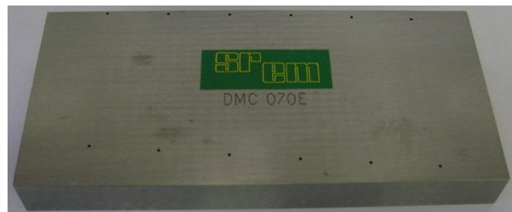
The reference block SNECMA is an excellent way for inspection of the polarity of magnetization coil, and the efficiency of the longitudinal magnetization.
